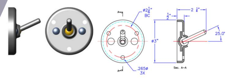
Construction Flang: 11 quage x 3" diameter type 304 stainless steel
